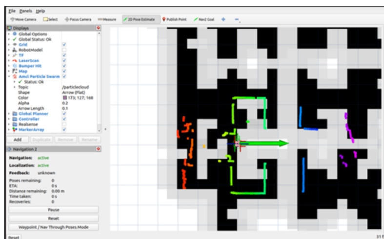
Figure 11: Robot localization process using 2D Pose Estimate feature in RViz2.
